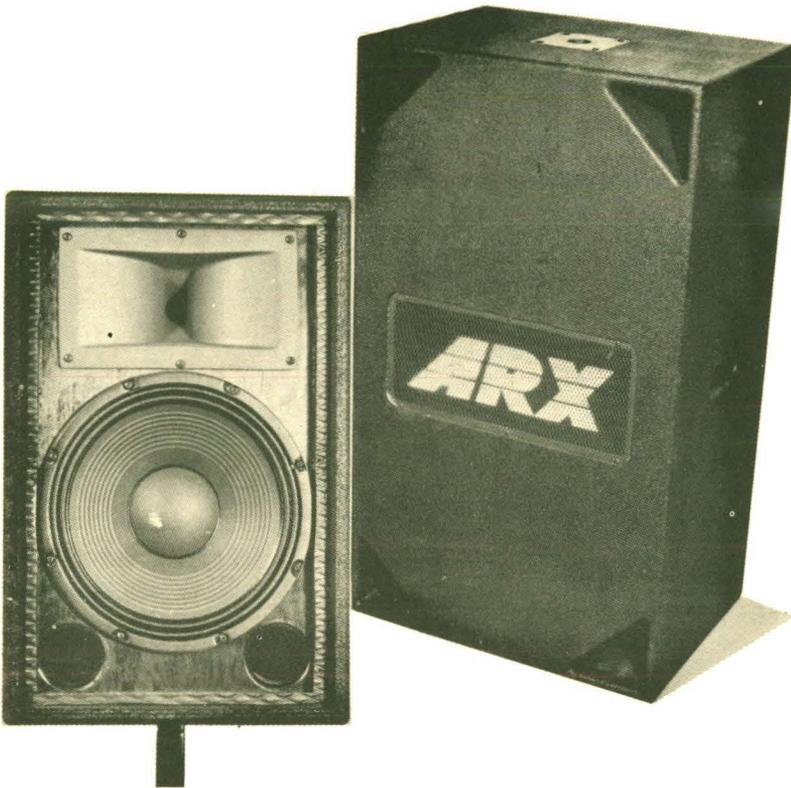
ARX has released a new series of compact, trapezoid, high SPL Loudspeaker Systems featuring state of the art passive crossovers. The PowerMax 1 full range loudspeaker features the ARX HPB12 High Excursion Low Frequency Driver & the EXF16 High Frequency Compression Driver. The PowerMax 1 utilises an all new Linkwitz Riley 24db Passive Crossover to ensure phase coherence through the crossover region.
