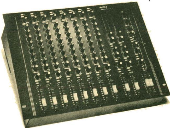
The Studio Server has been designed to offer features and quality in a compact package. Designed as an "Inline Console" it is available as a 8 or 16 channel rack mount and as a 24 channel free standing console. Features include 4 band EQ, 4 Auxiliary sends, 4 Stereo Line inputs and comprehensive master section. All three models feature the ability to switch Aux's 3 & 4 to input channels effectively giving you double the amount of inputs for mixdown. Many other features are easily
