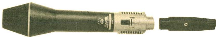
The D 202 uses the exclusive AKG Two-Way Technology: the bass (20-500Hz) and treble (500-20,000Hz) ranges are picked up by separate transducers, the result being a wide, flat frequency response. 3-step bass-cut (0, -7, -20dB at 50Hz); black plastic case.
