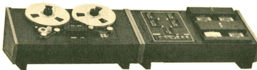
The 6120 XLP System boasts technical gains in frequency response distortion and cross-talk specifications. The new cassette transport speed allows you to duplicate directly from a 15 IPS reel master tape. A frequency response (+ - 3db) reel to cassette and cassette to cassette - 50 Hz to 30 kHz. Bias frequency reel 800kHz, cassette. 600kHz. Record level within 2db of master at 1kHz with level control in present position.
