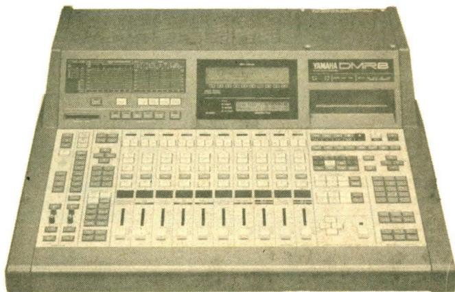
The DMR 8 is an integrated, all digital system for audio recording and mixing, with an 8 track digital recorder, digital mixer, locator, and mixing automation integrated into a single unit. It is intended for personal use by musicians, composers, and arrangers involved in commercial music production.
