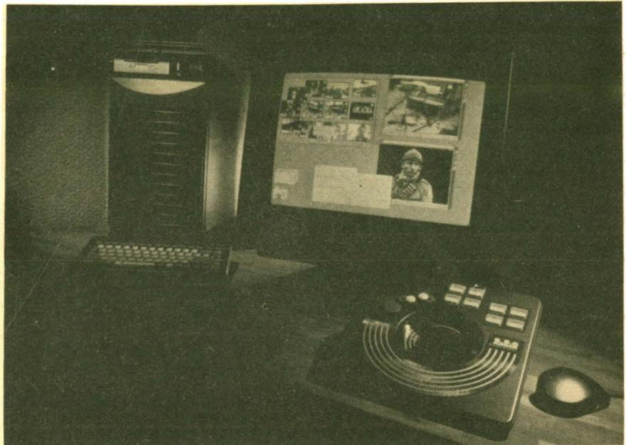
**Output:** The primary outputs of the system are editing decision lists and for video can be in any of the common standards. The system is supplied with 3 1/2" floppy disk drive but other sizes can be added.
