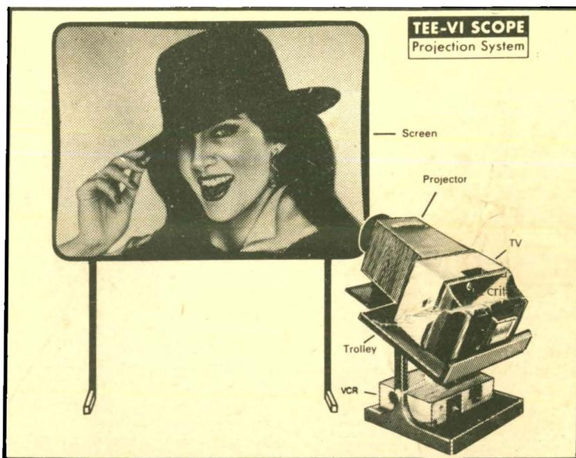
Magnascope – a TV enlarger. It is optically designed to magnify a 14"/20" TV or video image to 30" without any loss in clarity, brightness or sharpness. It is maintenance
