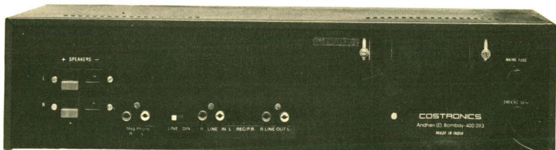
switched, the red LED glows in the centre of the face plate. The machine operates from 160 to 260 VAC mains supply which means it has high regulation. This feature is very good for rural areas or some cities in India where there is large AC voltage fluctuations. When
